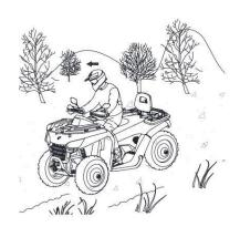
Driving on a sidehill is not recommended. Improper procedure could cause loss of control or overturn. Avoid sidehilling unless absolutely necessary.
