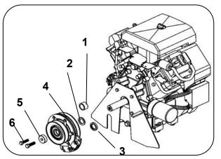
Mounting components of the electromagnetic clutch
