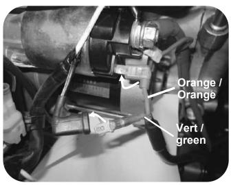
Connect cables of engine starter
