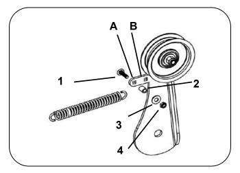
Adjusting the tension on the belt
