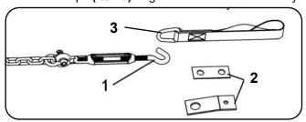
Installing the turnbuckles on the vehicle
