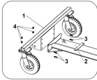
Installing the wheel support
