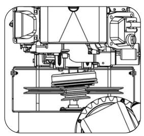
Angular pulley alignment error
