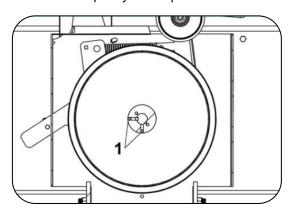
Remove the V pulley
