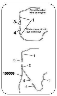
Connecting the engine circuit breaker wire
