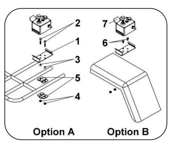
Installing the control box
