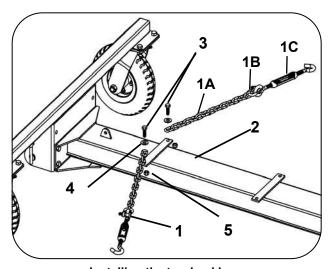
Installing the turnbuckles
