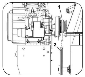
Parallel pulley alignment error
