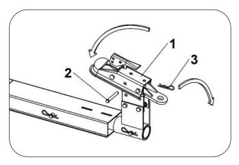
Installing the subframe on the tow hitch ball
