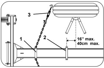
Installing the turnbuckles
