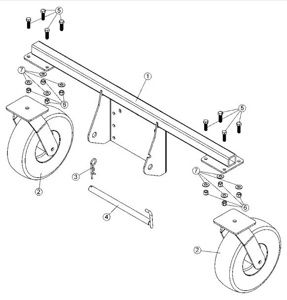
NOMENCLATURE ET LISTE DES PIÈCES / PARTS BREAKDOWN & PART LIST Souffleuse à Neige 48" VTT / VU "Versatile Plus" assemblé #501474 Snowblower 48" for ATV / UV "Versatile Plus" assembly #501474 1.6 25 (15) (22)
