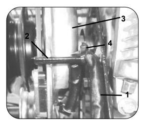
Connect wire to electromagnetic clutch
