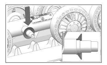
Apply evenly 3 to 3.5 cc of grease all around the wheel seal's V-shaped groove.
