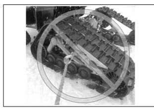
CAUTION: The towing cable must be attached to the vehicle's frame.
