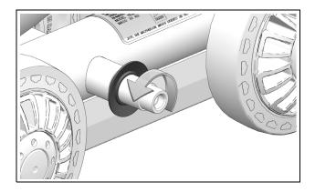
Unbolt wheel from frame and carefully remove exterior bearing seal (1) of both bearings. Clean off old lubricant and pack with new grease. Lastly, re-install seals over matching bearings.
