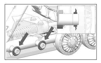
Apply evenly 3 to 3.5 cc of grease all around the wheel seal's V-shaped groove.
