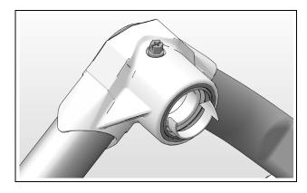
**IMPORTANT:** The hub seal must be installed flush with the hub face.
