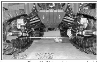
Figure 26 (Distance between rear wheels)
