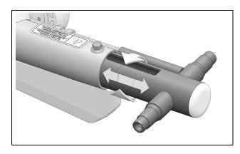
NOTE: Application of lubricant on the tensioner tubing prevents corrosion inside the frame. Lubrication allows the tensioner to move freely when adjusting the track's tension.
