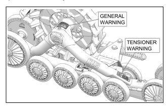
CAUTION: Do not remove the warning sticker from the frame. If a sticker is damaged, have it replaced at an authorized Camso dealer.
