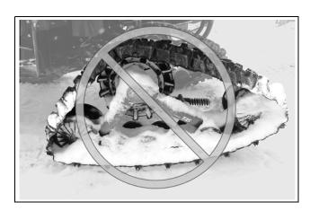
CAUTION: Track systems installed on an ATV or SxS project more snow, dirt, water, or mud than tires. The owner/driver is responsible for adapting engine and CVT air intakes to minimize the risks of breakdowns and/or damage to mechanical components.
