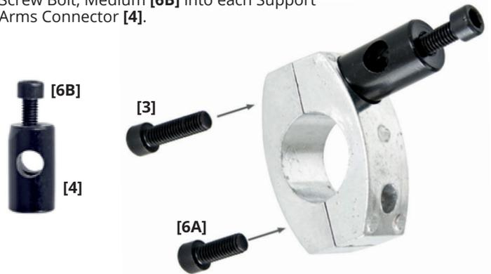
**#3** Install Windshield support arm [5] into each Support Arms Connector [4] and fix it with Bolt, Medium [6B].
