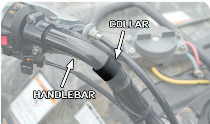
**#2** Install Handlebar clamp [2] over the Plastic collar [1] using Bolt, Short [6A]. Place Support Arms Connector [4] into the recessed hole of the Handlebar clamp [2], and screw it through the Clamp using Bolt, Long [3]. Screw Bolt, Medium [6B] into each Support Arms Connector [4].
